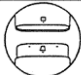
JOINING OVAL FITTINGS Fig. 1 - To join, push upper section down onto lower section until "Fastloc" tabs are engaged.
